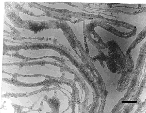
Figure 2. Transmission electron micrograph of "shish kebabs" of i-PS prepared from 0.01 wt % solution containing self-nuclei, crystallized at 175 °C for 8 h. 100 \mu L of solution was added onto the water surface. The scale bar indicates 500 nm.
